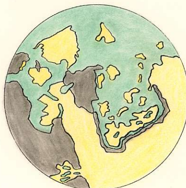
Core Replacement of hornblende crystal by chalcopyrite. Note rim reaction in B. Rim is quartz, protecting hornblende (Text: p 19)
