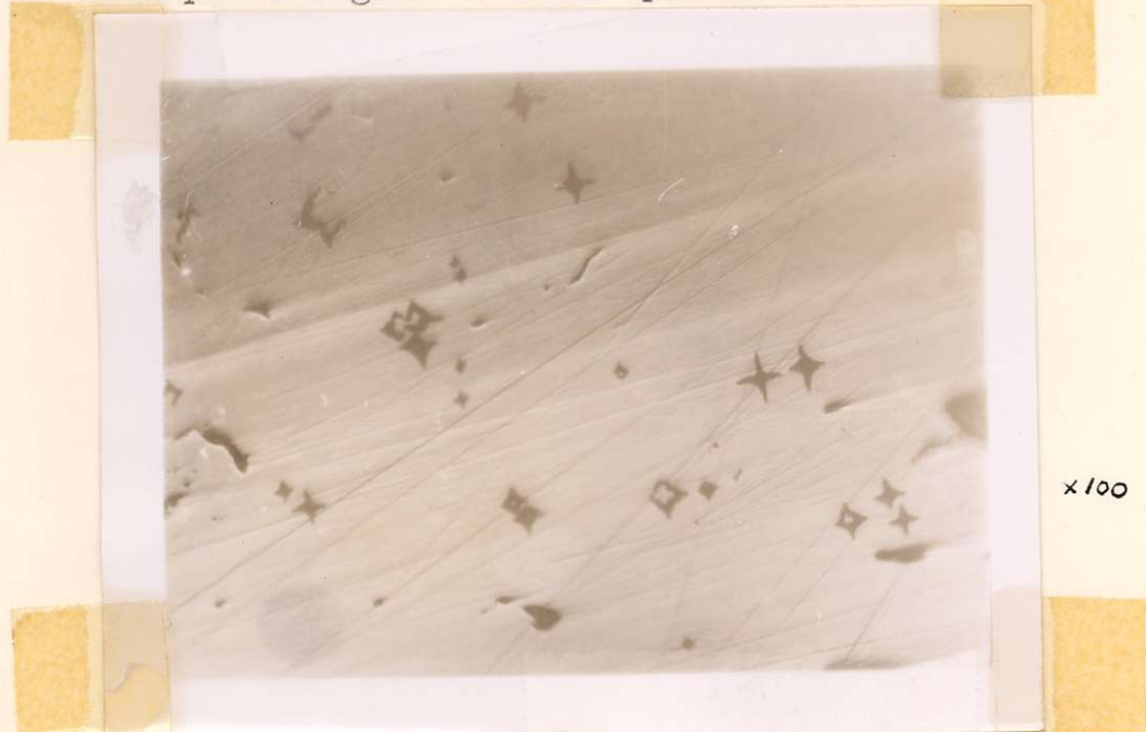
SPHALERITE STARS (DARK) IN CHALCOPYRITE (LIGHT)
