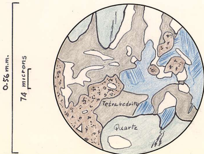
FIG. 5 GALENA REPLACED BY TETRAHEDRITE AND BOURNONITE. ROUNDED AND ANGULAR INCLUSIONS OF GALENA IN SPHALERITE. POLY- SYNTHETIC TWINNING IN BOURNONITE.
