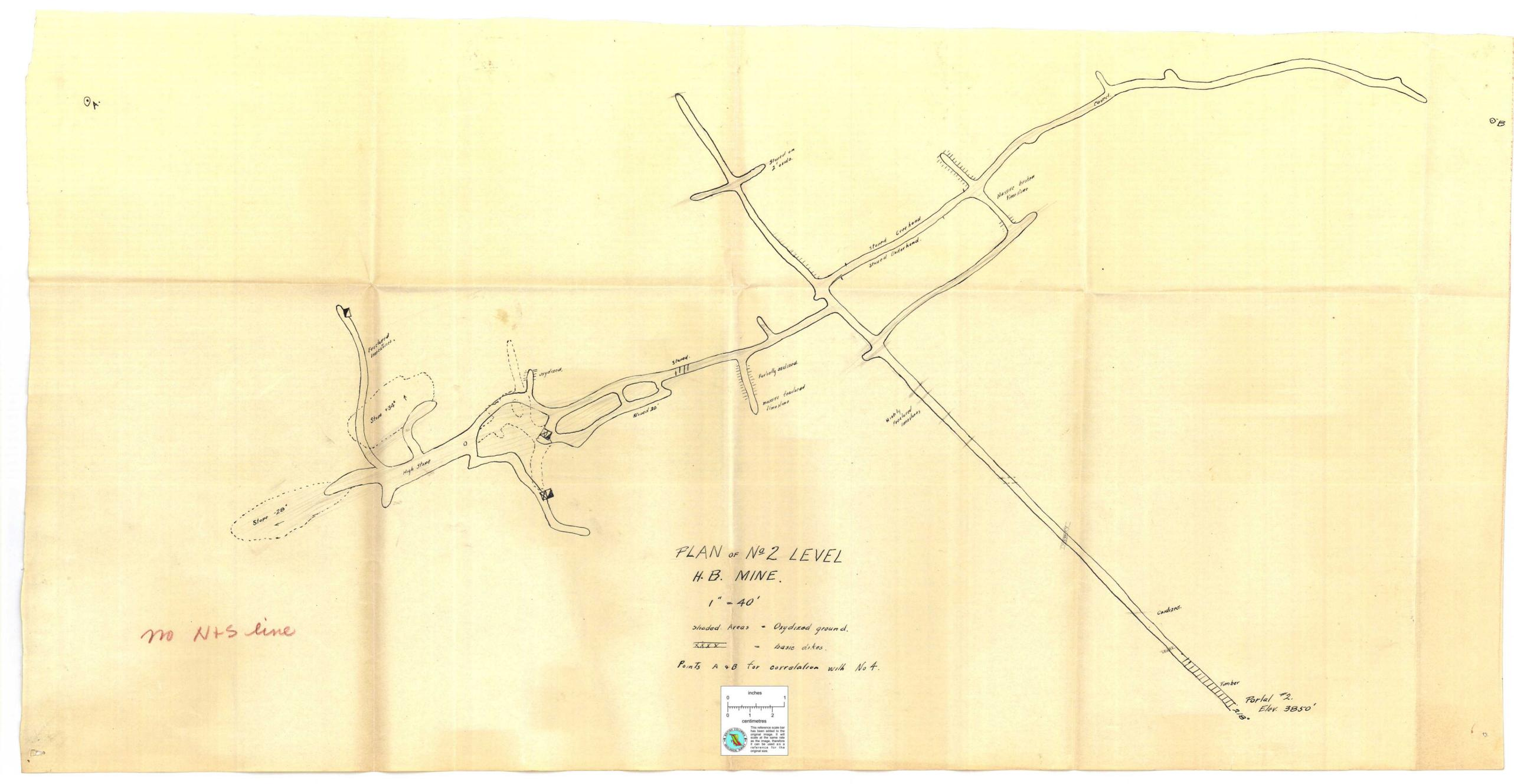
Nº. 4 Level. H.B. Mine. Scale 1" = 40' Points A & B for correlating with Nº2. 0 A XXXX dikes slips. Limos lom. Fractoried Highly Fraclared Limestones Oxidized\_ (--Fraelurod Limeslones 0 Z P Z • Massive Fractured Ls. Sev.
