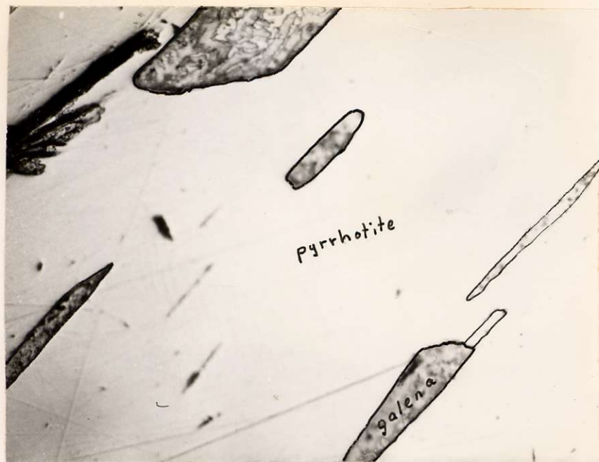
Fig. 9. Replacement of pyrrhotite by galena along cleavage planes
