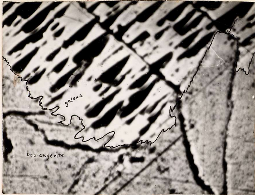
Fig 7. Replacement of galena by boulangerite.
