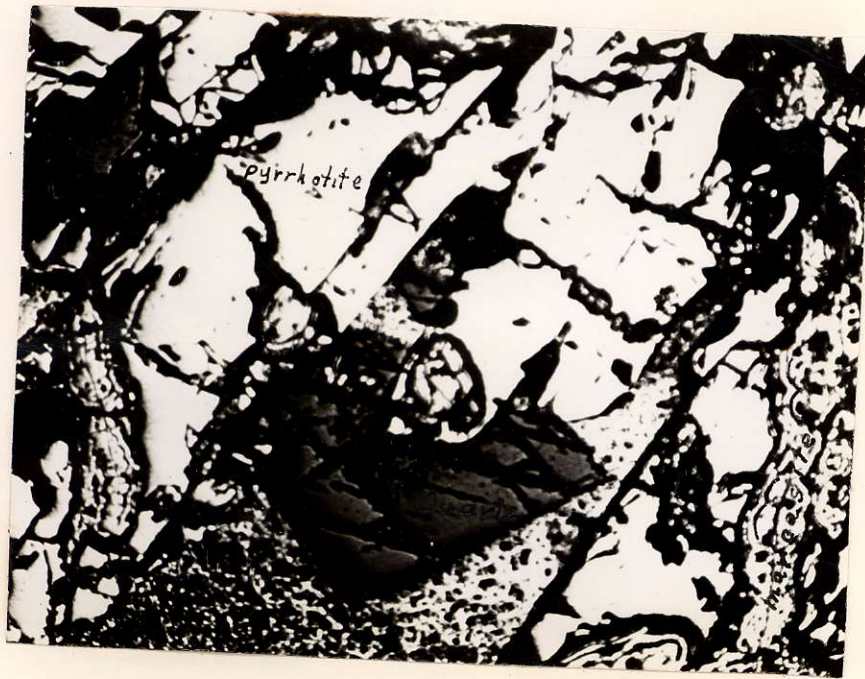
Fig 6. Alteration of pyrrhotite to marcasite.
