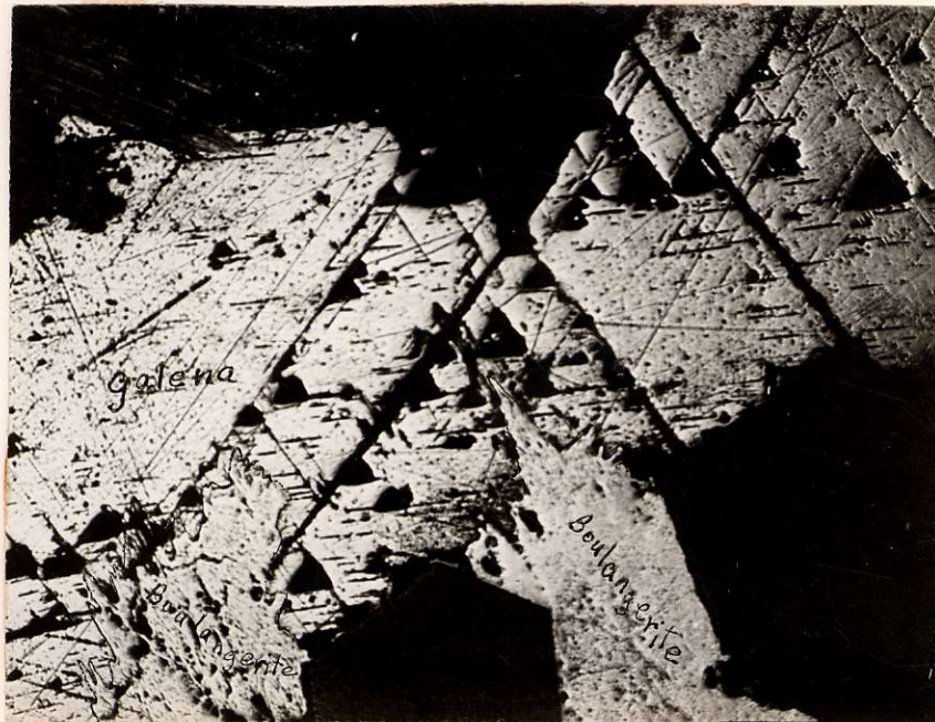
Fig. 8. Fibrous boulangerite replacing galena
