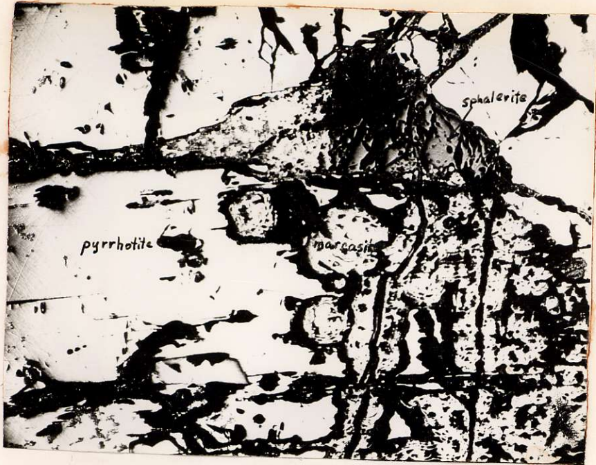
Fig 3. Alteration of pyrrhotite to marcasite along fractures
