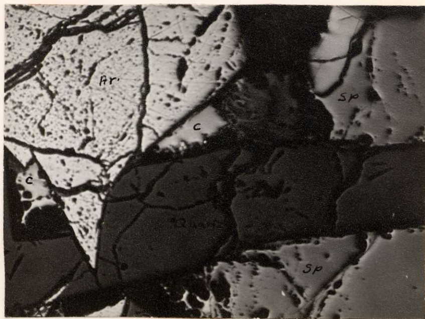
Fig. 10. Boundary relations of arsenopyrite (Ar) Chalcopyrite (C), sphalerite (Sp) and cut by quartz vein (dark grey)
