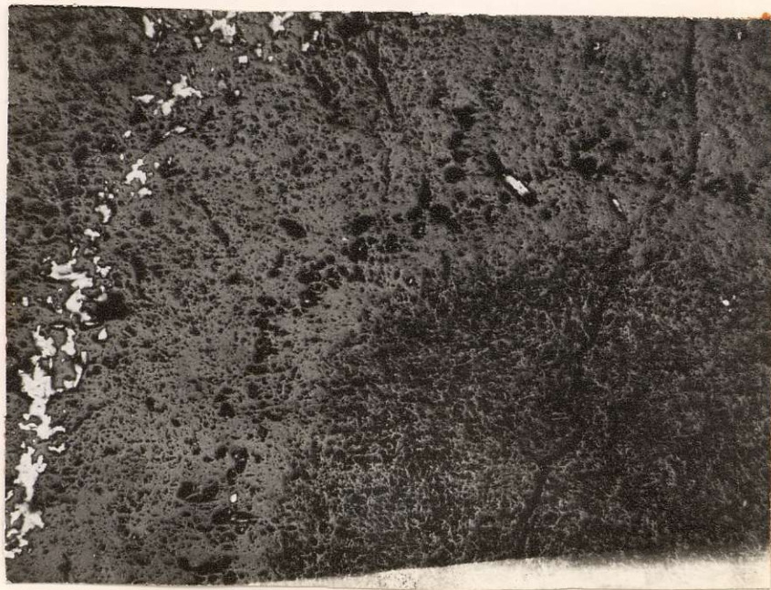
Fig 14. Siderite growth rings surrounded by Jamesonite(?)
