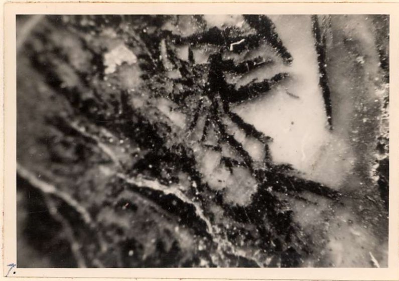
Plate 7: Showing feathery projections of sphalerite (dark) into gangue (white). Reflected, oblique light. Magnification: about 50X
