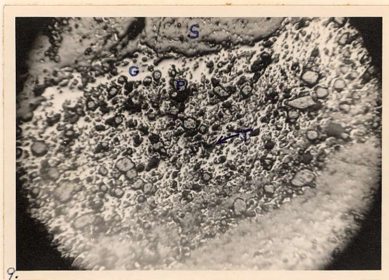
Plate 9: Photomicrograph showing galena (G) invading sphalerite (S) and containing fragments of sphalerite, pyrite (P) and tetrahedrite (T). Magnification: 30X
