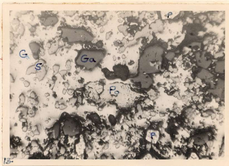
Plate 13: Photomicrograph showing polybasite (?) (Po) in galena (G). S is sphalerite; Ga, gangue; P, pyrite. Magnification: 140X.
