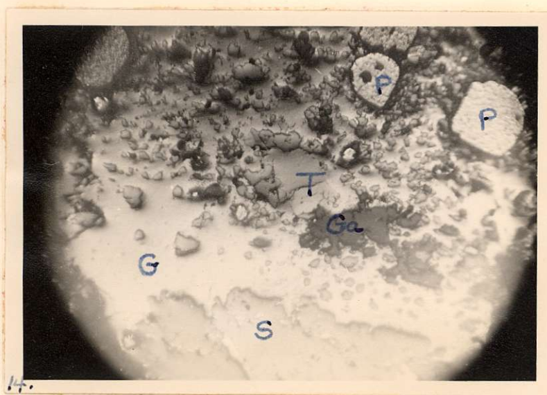
Plate 14: Photomicrograph showing tetrahedrite (?) (T) in galena (G). S is sphalerite; P, pyrite; Ga, gangue. Magnification: 70X
