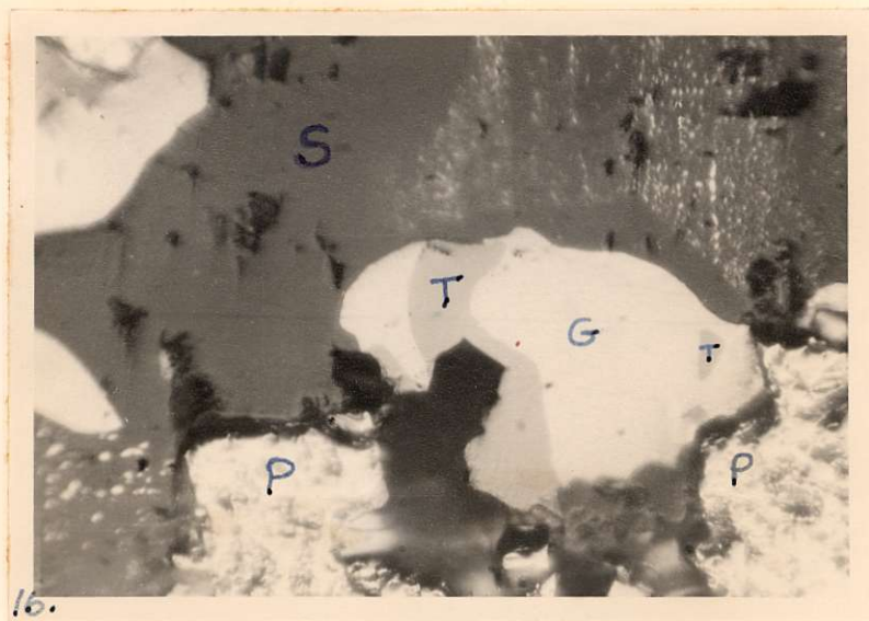
Plate 16: Photomicrograph showing bleb of tetrahedrite(?) (T) in galena (G). S is sphalerite; P, pyrite. The mass of light specks in the sphalerite in the lower left-hand corner of the photo is chalcopyrite. Oil immersion. Magnification: 670X
