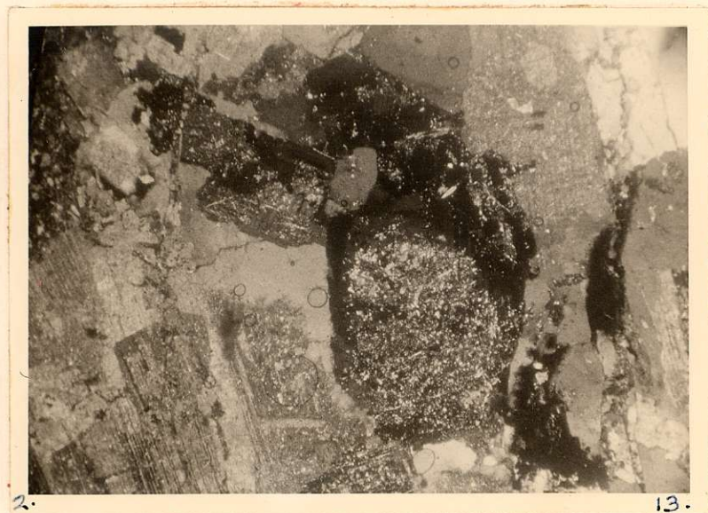
Plate 2: Photomicrograph with crossed nicols showing alteration (particularly, sericitization) of the feldspars, particularly the plagioclase. Magnification: 70X
