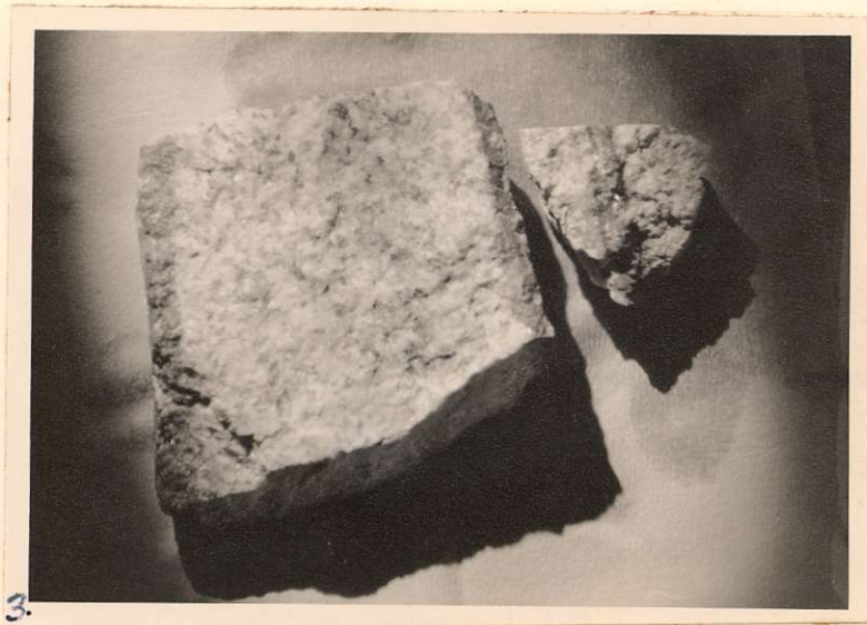
Figure 3: Showing two specimens of granodiorite; one containing a small galena vein. Large piece is about five inches across.
