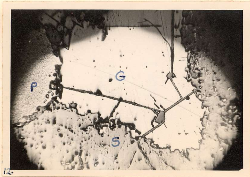
Plate 12: Photomicrograph showing galena (G) being replaced along cleavage planes by sphalerite (S). P is pyrite. White specks in sphalerite are galena and chalcopyrite the galena tends to have a dark border due to relief. Magnification: 30X.
