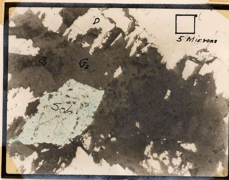
Figure 2: Section E, showing Danaite and Safflorite-loellingite replaced by one generation of quartz. Another generation of quartz is seen veining the first generation.
