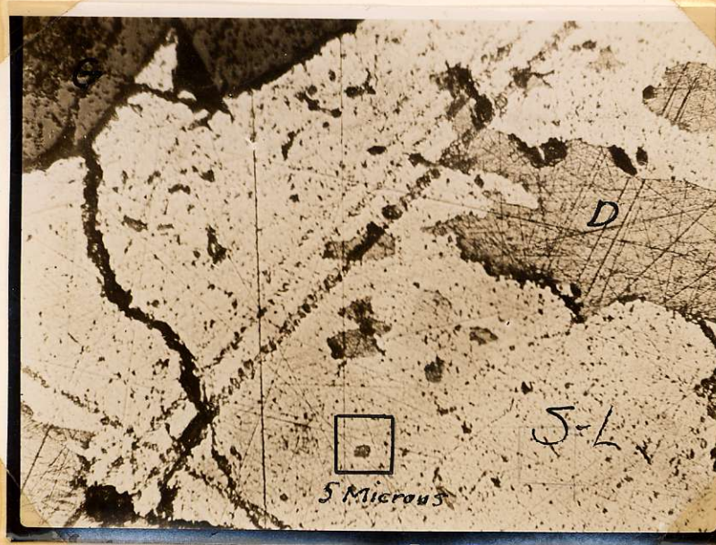
Figure 2: Section E, showing Danaite and Safflorite-loellingite replaced by one generation of quartz. Another generation of quartz is seen veining the first generation.
