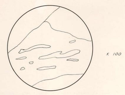
Diagram showing the parallel arrangement of the inclusions, after etching with FeCl
