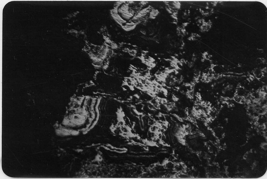
Figure 5 Alteration of pyrrhotite(core) to marcasite(concentric rings). Taken under reflected light and one nicol.
