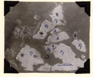
Description: Original shape of pyrite was triangular. It has been replaced by arsenopyrite and sphalerite chiefly and by galena in a minor extent.
