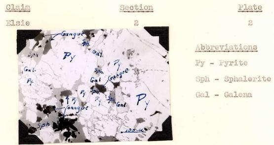
Description: Indication of age relations between pyrite, gangue, sphalerite and galena. This also shows to a minor extent the tendency for pyrite to be replaced along its cleavage planes - suggested by the rectangular pattern of the fractioning.
