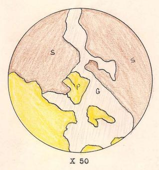
Section showing galena (G), veining sphalerite (S), and pyrite (P).
