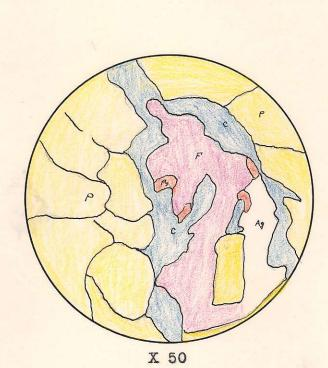
Section showing freibergite (F), pyrargerite (Py), native silver (Ag), and calcite (C), veining pyrite (P).
