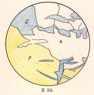
Section showing quartz (Q), veining pyrite (P), and arsenopyrite (A).
