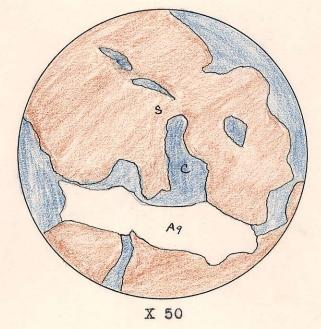
Section showing calcite (C), and native silver (Ag), veining sphalerite (S).
