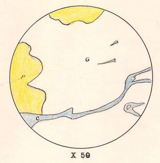
Section showing calcite (C) veining galena (G) and pyrite (P).
