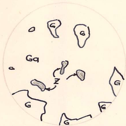
POLISHED SECTION No. 2 (B) SHOWING MINERAL "Z" IN GALENA (MAG X 120)
