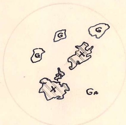
POLISHED SECTION No. 6(A) MINERAL X IN GALENA MAG X120
