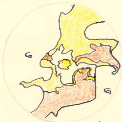
POLISHED SECTION No. BA (C) SHOWING EVIDENCE OF GALENA LATER THAN BORNITE & REPLACING CHALCOPYRITE PREFERENTIALLY TO BORNITE. (MAG X 120)
