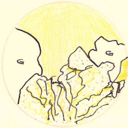
POLISHED SECTION No. 8B(B) SHOWING CHALCOPYRITE LATER THAN PYRITE & FILLING FRACTURES IN PYRITE MAGXIZO
