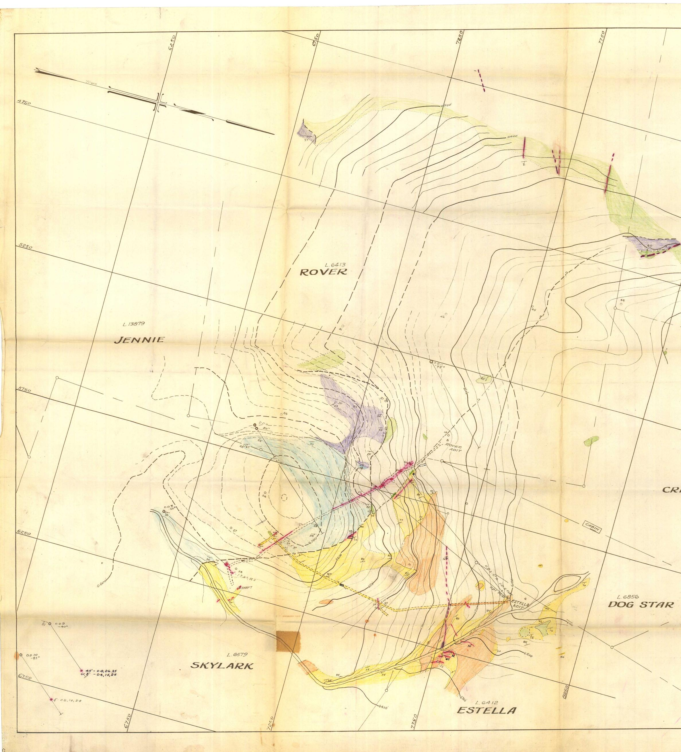
6000---- 6000 <u>ESTELLA MINE</u> FORT STEELE M. DIV. B. C. SCALE: linch= 100 feet 0 1 2 centimetres This reference scale ba has been added to the original image. It will as the image, therefore is can be used as a original size. L.6854 VIKING L. 6853 CRESCENT L. 13880 DOLLY Porphyritic Syenite Diorite; greenstone. On sections diorite has X X Aldridge-Argillite-siltstone. Fort Steele - Argillite-Siltstone. . 32 Uncorrelated argillite etc. of footwall. Veins.
