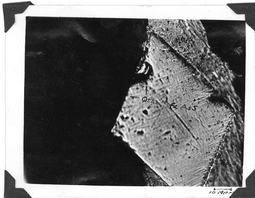
Fig. 1 (x780) Showing stibnite replacing quartz and arsenopyrite and quartz replacing arsenopyrite.
