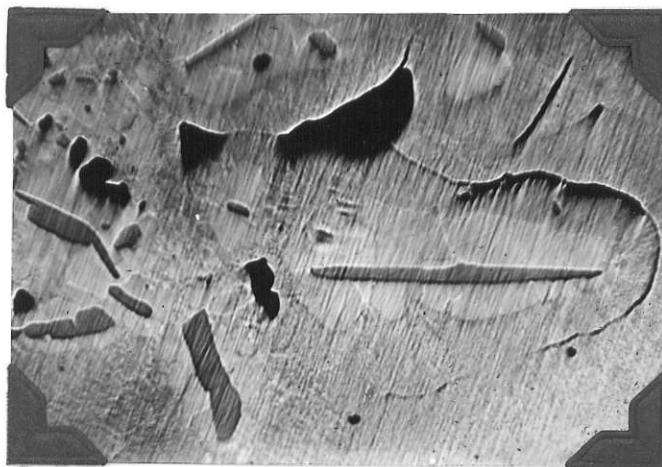
Fig. 7. From specimen MgA-1, Mag. X75 Dyscrasite - nearly black laths (tarnished with \text{HNO}_3 fumes) Allemontite - grey areas surrounding dyscrasite Arsenic - dark grey groundmass Holes - black
