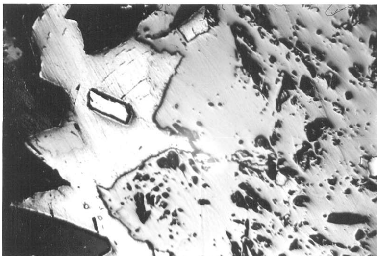
X150 Galena (light) replacing sphalerite (dark). The light lath-like grain is arsenopyrite.
