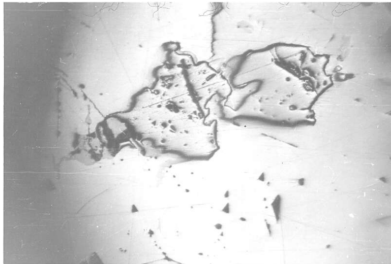
X150 Corroded pyrrhotite grain sitting in galena.
