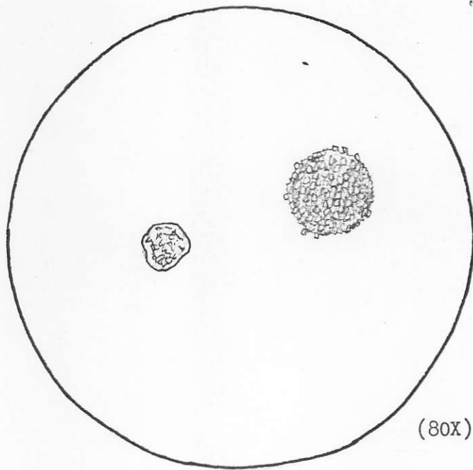
SKETCH 1 : Framboidal pyrite (yellow) showing structure of hundreds of minute cubes. Note spherical shape of framboid. (from polished section Alcock #1).
