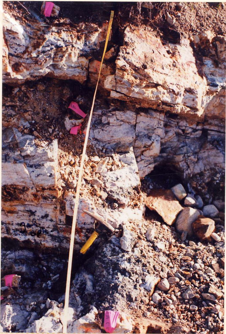
VEIN A - galena, sphal, cpy - banded.
