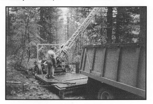
Although the Eureka has NEVER been drilled, I thought I'd put in a picture of our Boyles portable Diamond Drill that is capable of drilling up to 500ft. NQ and 700ft. BQ and is readily available at very reasonable prices.
