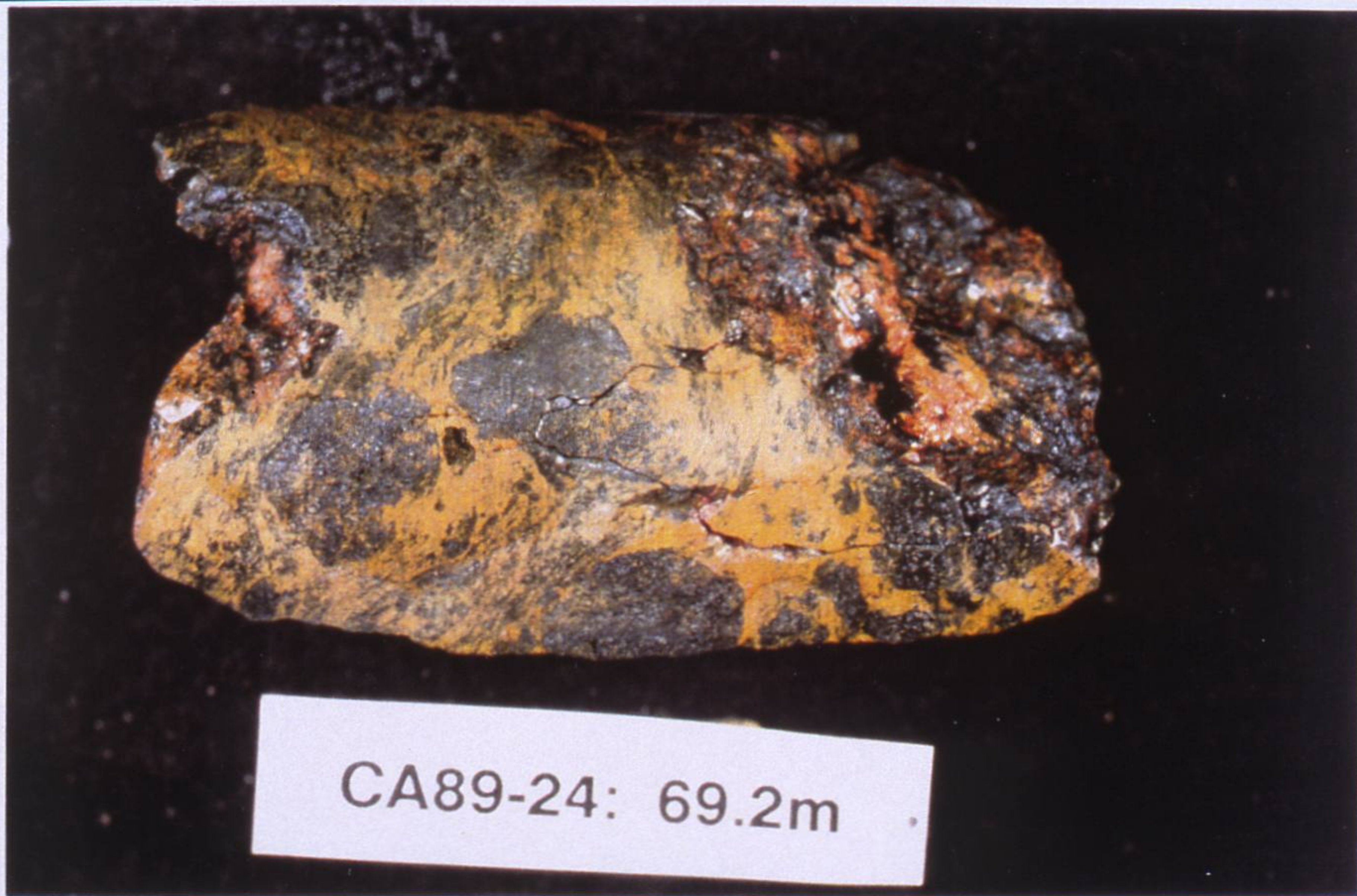
Figure 4.22: Clasts of stibnite with minor realgar hosted in a matrix of realgar with minor stibnite. (Core size is NQ).
