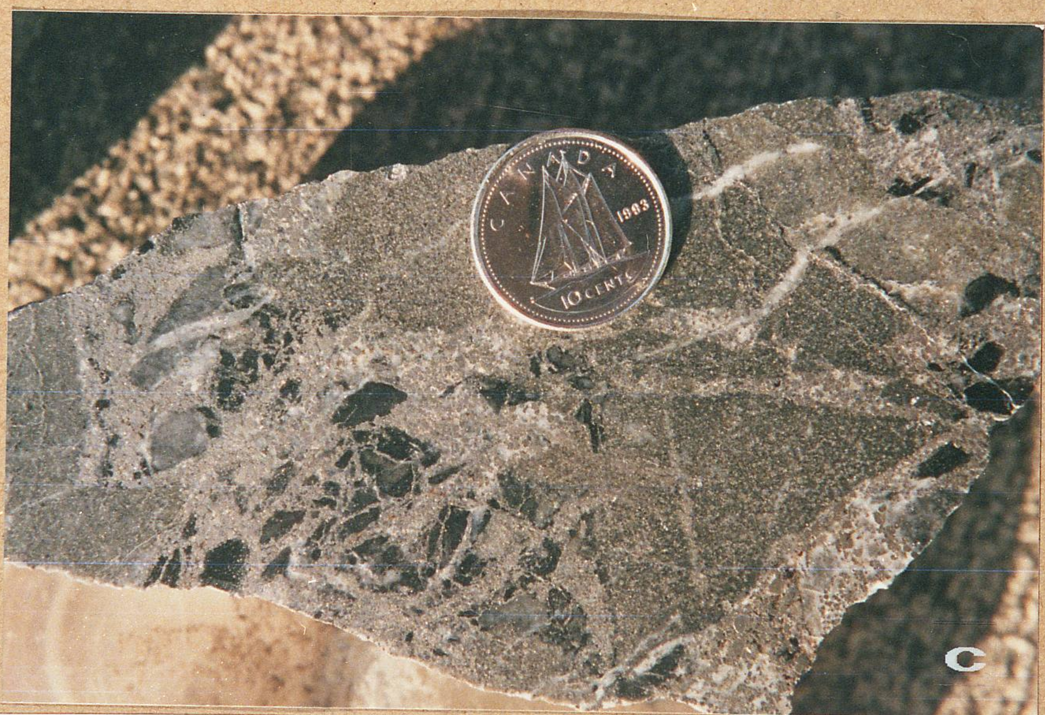
Cut and polished samplpes from the Marc zone: a) HIGH GRADE (5 - 6 opt Au)! massive coarse-grained (recrystallized) pyrite; b) mineralized Hillside porphyry: massive coarse-grained pyrite-quartz vein plus fracture-hosted and disseminated pyrite, Marc zone; c) mineralized heterolithic breccia: medium-grained pyrite is disseminated in matrix and angular fragments of Hillside porphyry and argillite-siltstone.
