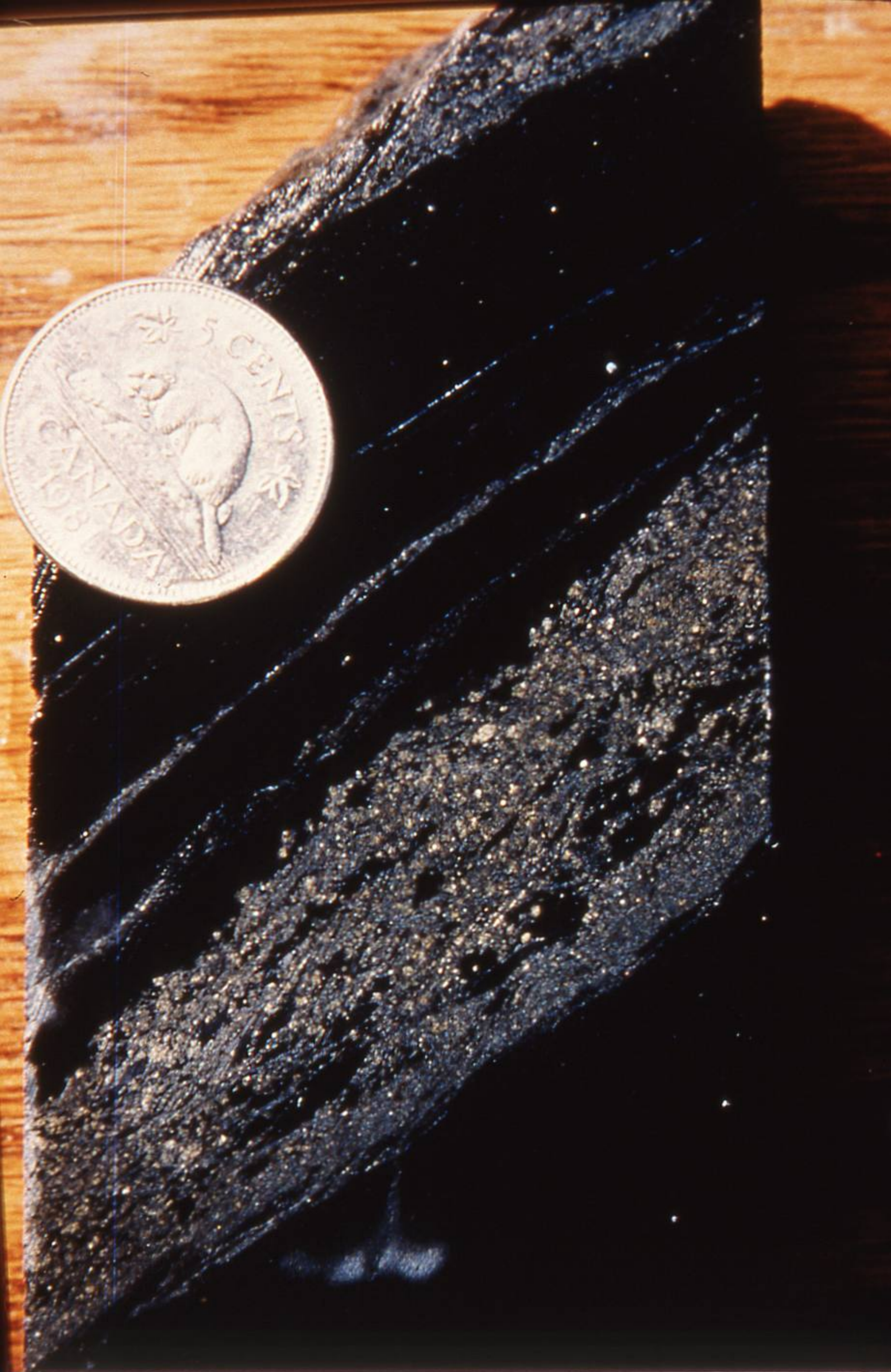
Massive sulphides (sphalerite, tetrahedrite, boulangerite, bournonite) in mudstone, Contact Unit, 21B Deposit, Eskay Creek, DDH CA89-86: 82.5m.
