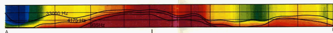
AERODAT RESISTIVITY - DEPTH SECTION - LINE 10070 935, 4175, 33000 Hz resistivity vs. centroid depth
