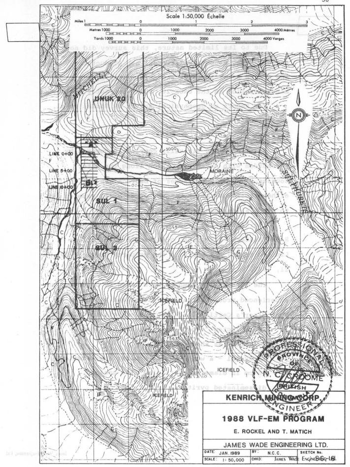
Due to its limited nature, this survey did not establish any geophysical trends. but Conductors A and B (see SC-6) indicate the possibility of sulfide mineralization on the UNUK-20, SUL-1 and SUL-2 claims.
