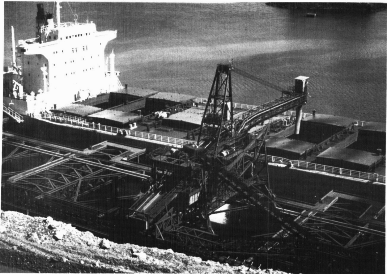
(Wesfrob Mines Limited - Tasu, B. C.) Figure 7 - Shiploader loading iron concentrate aboard M. S. Jasaka.
