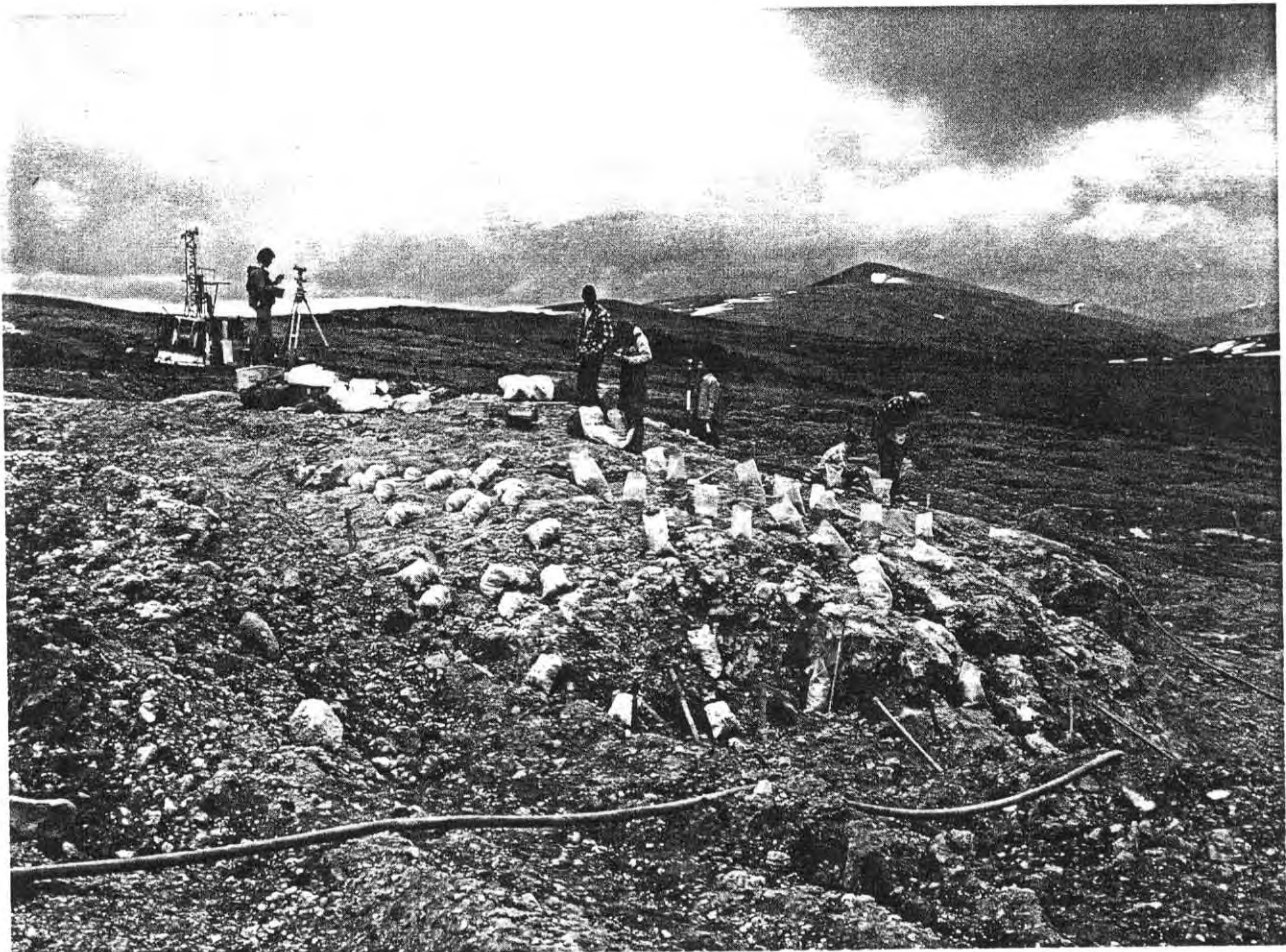
Detailed Channel Sampling, Proposed "A" Zone Pit, Thesis III Deposit
