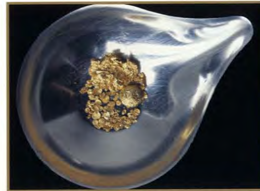
Gold beads and button generated in the fire assay process at Kemess
