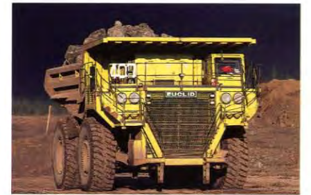
The primary haulage equipment at Kemess is the Canadian-made Euclid R260 truck. Tire life on each of the 13 trucks in the fleet has been doubled since Northgate acquired the mine.
