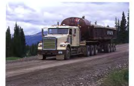
Specially designed trucks haul concentrate from the Kemess South mine to the railhead at Mackenzie and backhaul fuel and grinding steel to the mine site.
