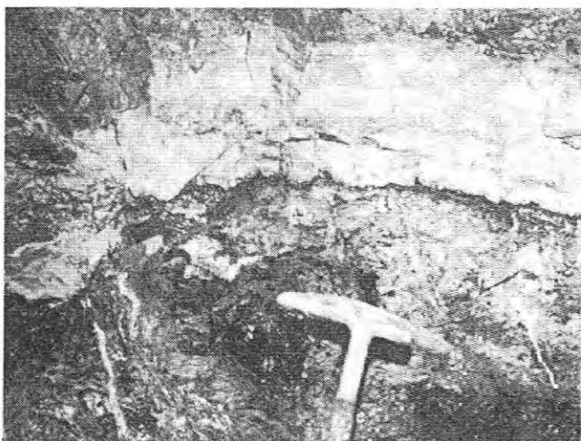
Fig. 11d — Banded part of vein against chloritized hanging wall in 5420 drift (coin diam. 1.75 cm).
