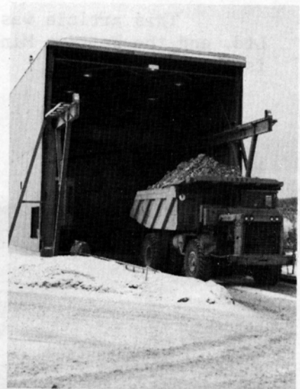
Granisle: about to dump into the primary crusher
