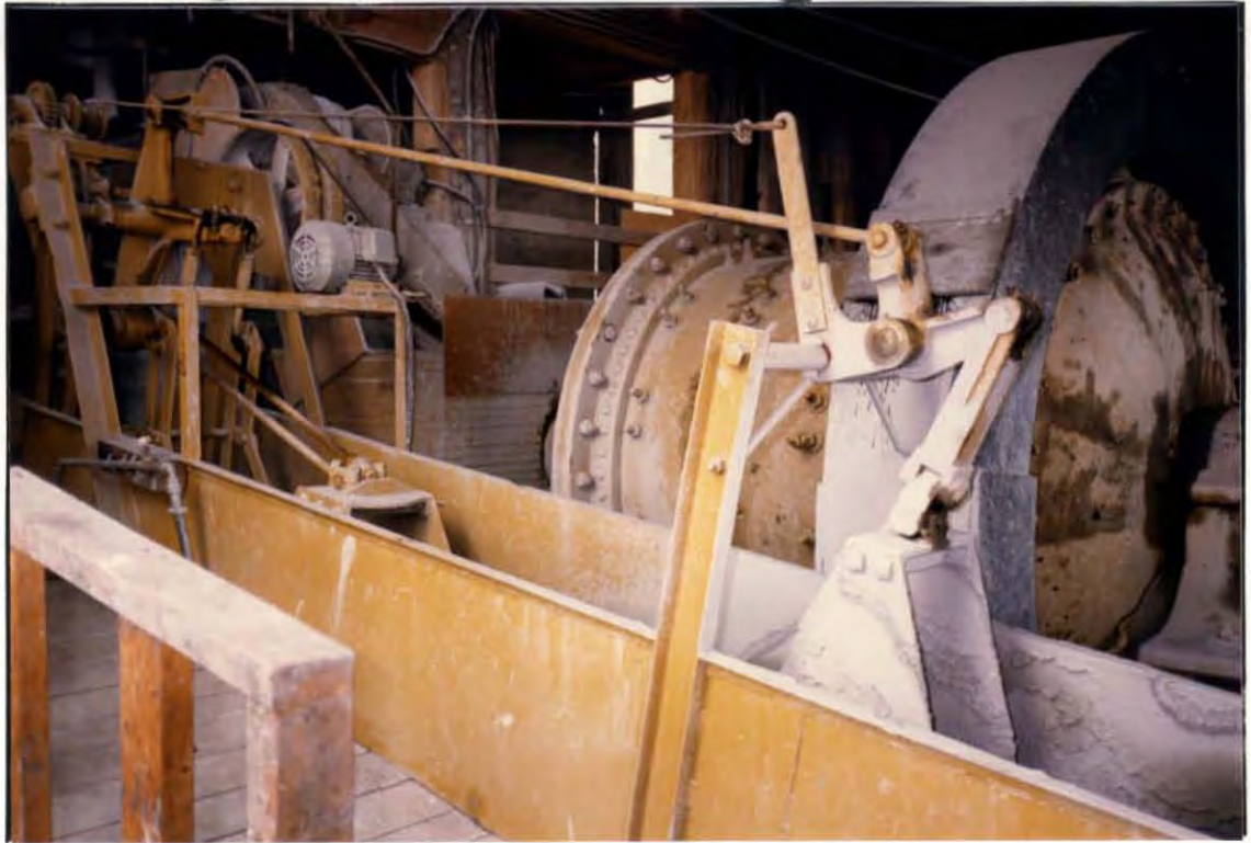
86-Roll 4 - 2 Feed goes directly into a ball mill with automatic recycling until it is pulverized to a fine powder.
