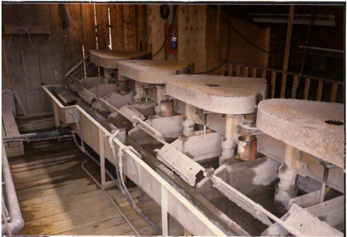
86-Roll 4 - 3 Eight flotation cells are used to separate concentrate.
