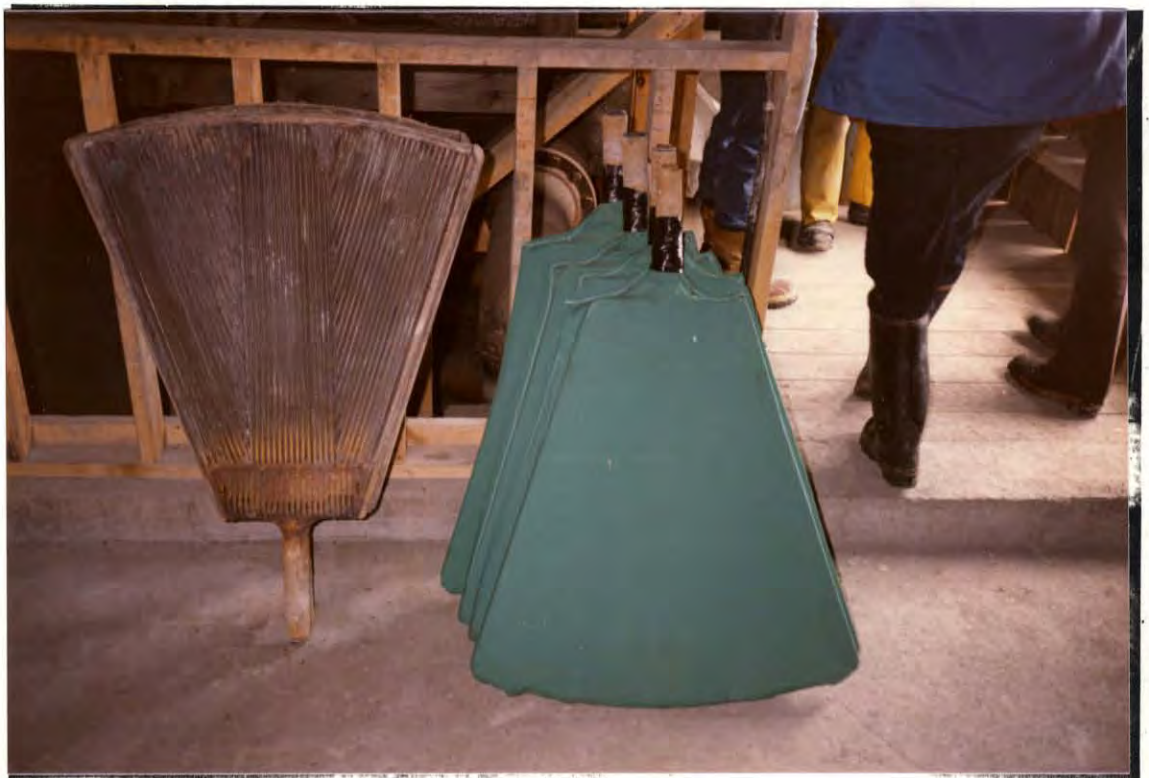
86-Roll 4 - 4 After much experimentation with the disk filters, Paul Kindrat has found that material (green) bought in town for $6 is more effective than the prefitted $25 bags used by Equity Silver Mine.
