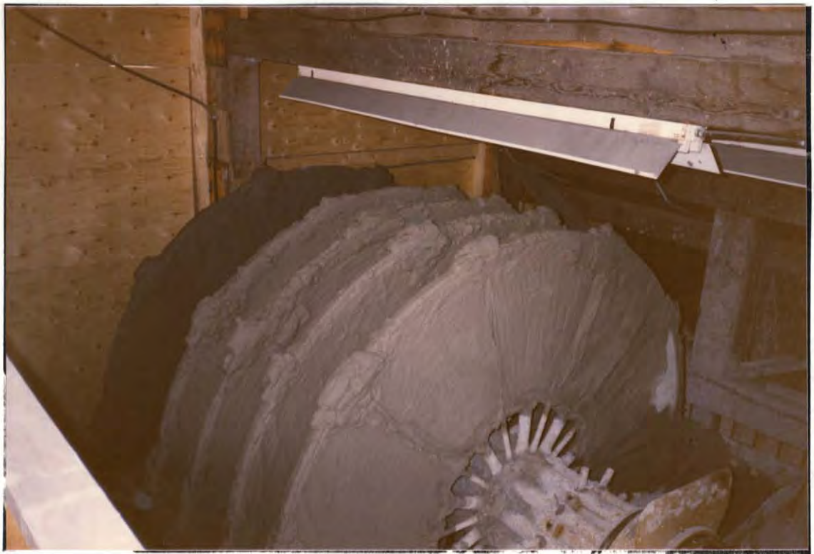
86-Roll 4 - 5 Four disk filters are used - dark one for ore concentrate and three light coloured filters for tailings. Mill is a closed circuit with water being recycled and dry tailings.
