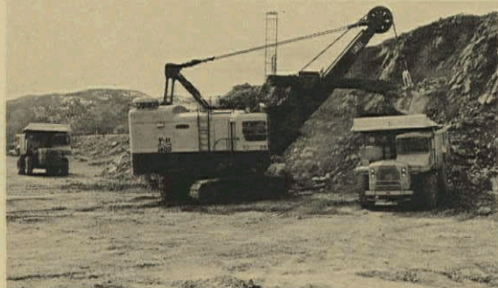
An electric shovel in the open pit loads 5 cubic yards of ore into a 35 ton truck. Behind is the mast of a 9" rotary drill.
