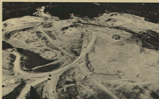
The open pit area with waste dumps and stockpile areas lower center and to left. Mining area, center.
