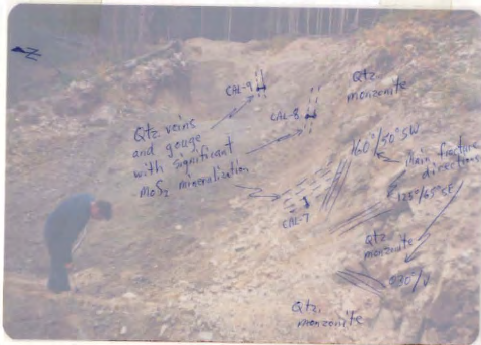
Trench on CALEDONIA property showing good fracture density (3 directions mineralized) and good mineralized quartz veins and gouge.
