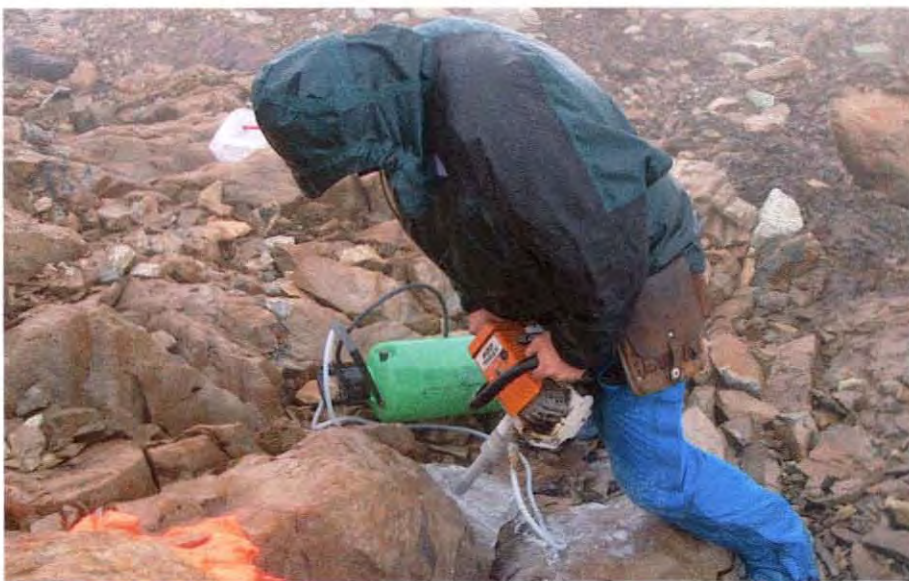
Aug.21, 2001 - Brian taking Paleomagnetic Cores at Saloomt Pk.
