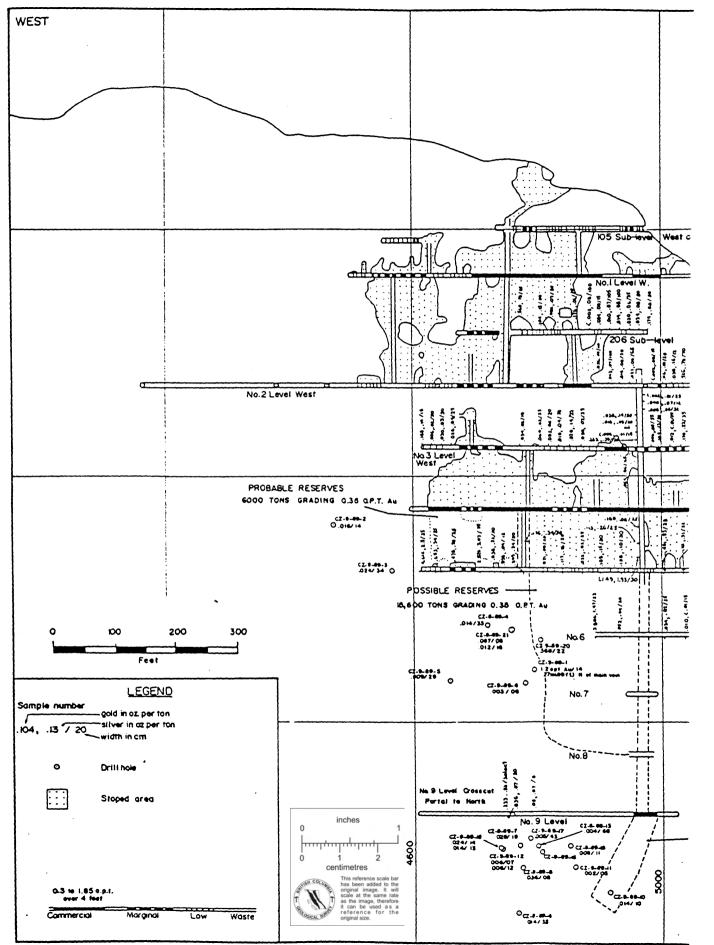
Drill hole No.s CZ-9-88-1 to 89-6, 20 and 21 tested the downward extension of the ore shoots blocked out on the No.5 level and indicated by recent sampling at the western face of both the No. 5 and 6 levels. At the same time the narrower veins paralleling the main vein to the north were also tested by these holes.
