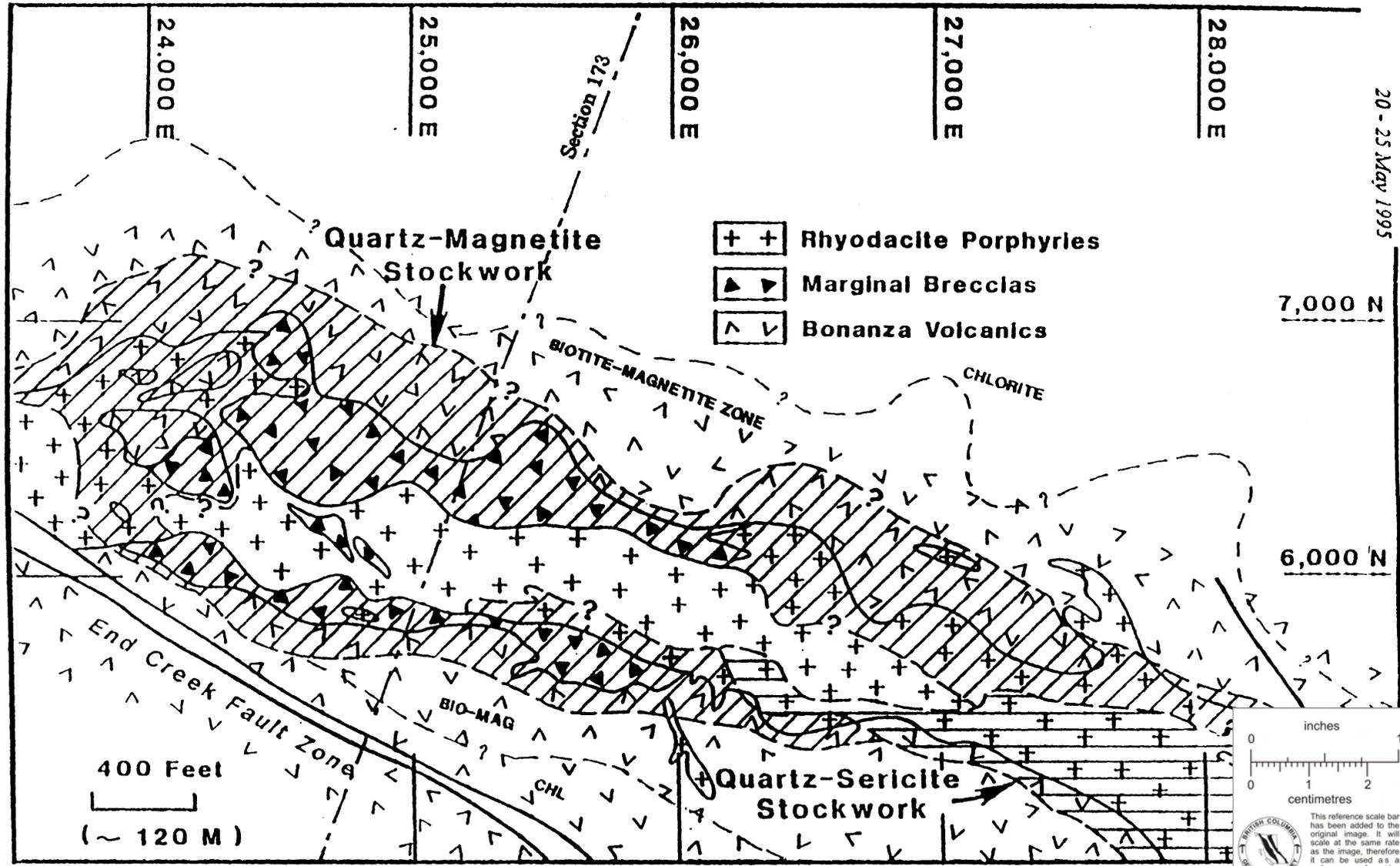
Figure 13. Detailed geology of the 560 bench, Island Copper mine, northern Vancouver Island.
