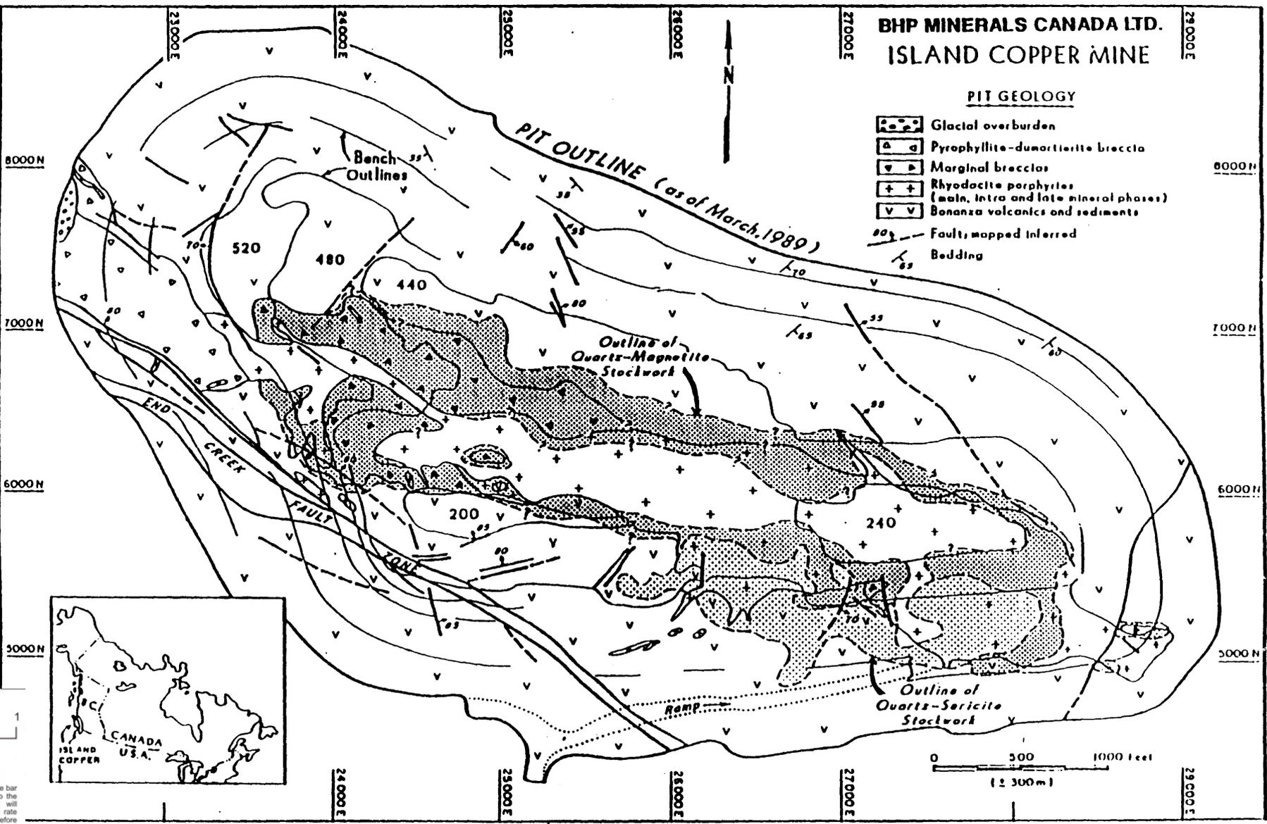
Figure 12. Pit plan geology (March 1989) of the Island Copper mine, northern Vancouver Island
