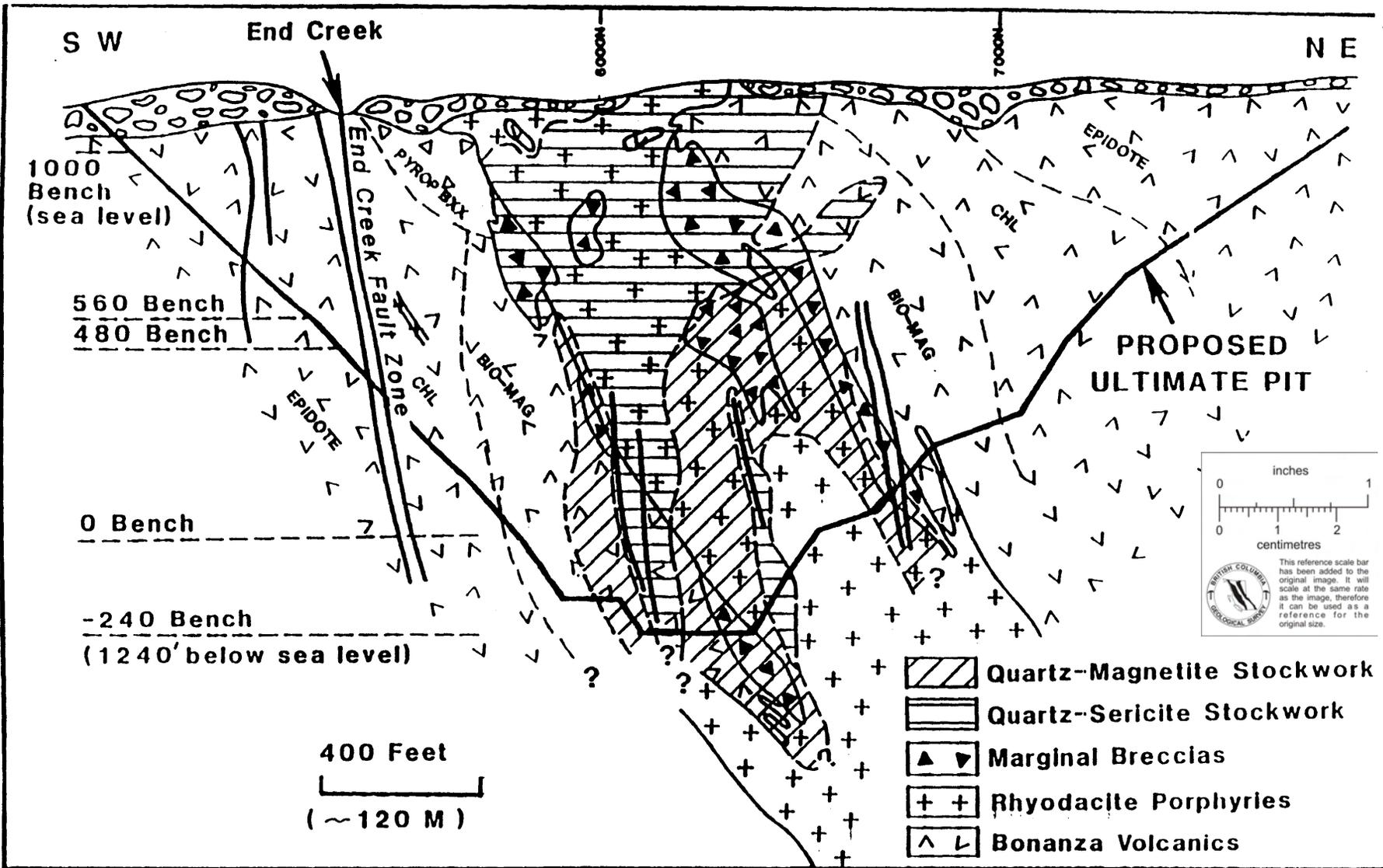
Figure 14. Detailed geology of section 173 west, Island Copper mine, northern Vancouver Island.
