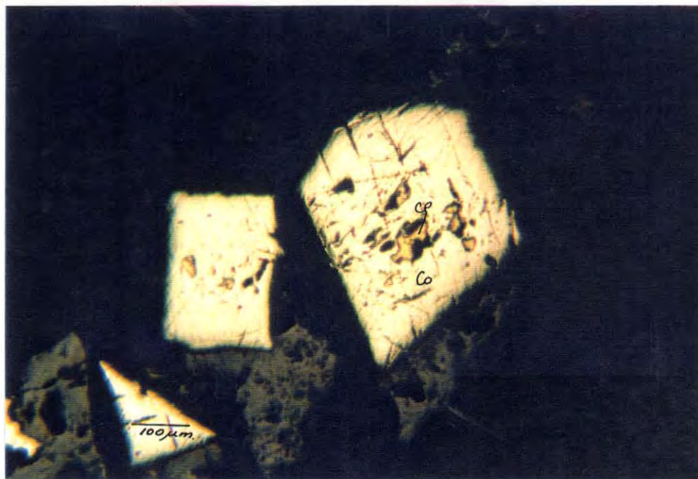
Plate 6: Cobaltite with chalcopyrite poikiloblasts. Sample MW Raven Copper 1.
