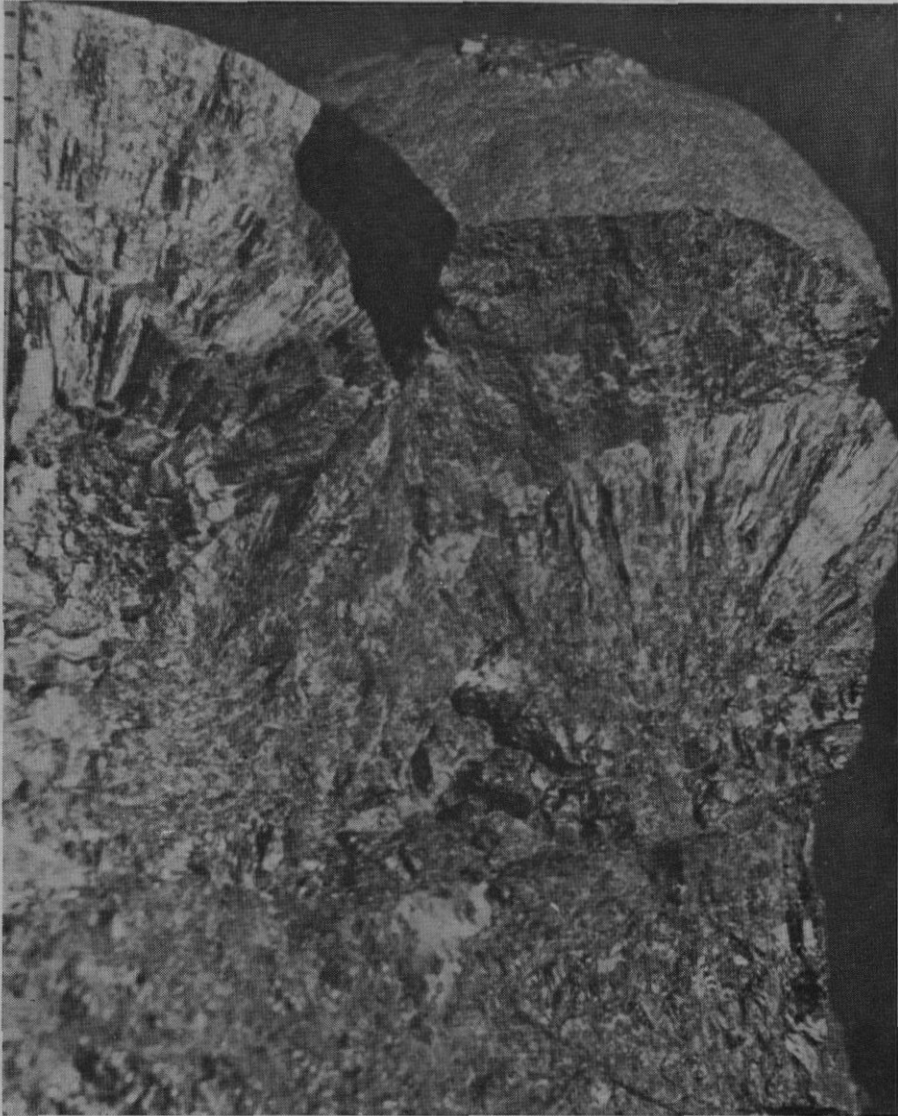
FIG. 2. Specimen of colloform magnetite broken to show internal radial structure. Specimen 3 inches across.
