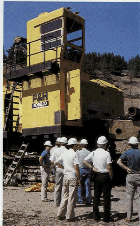
One of two P&H 1600 electric shovels being inspected by company directors. This mammoth equipment is used for loading ore in the pit area
