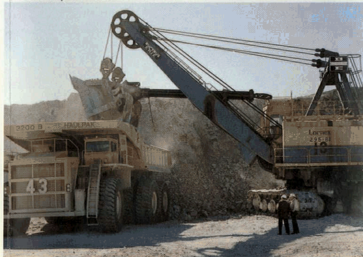
▼ A 22-cubic-yard shovel loads a 235-ton truck
