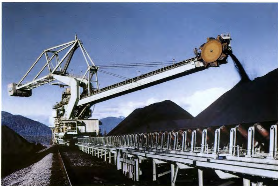
One of two coal stacker-reclaimers at the Ridley Island coal port, Prince Rupert, British Columbia.
