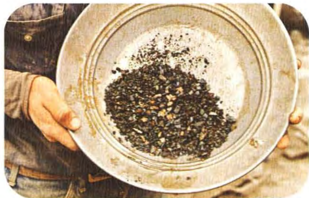
Native copper from a typical rotary drill hole. The fragments were concentrated in this gold pan to demonstrate some characteristics of the mineralization
