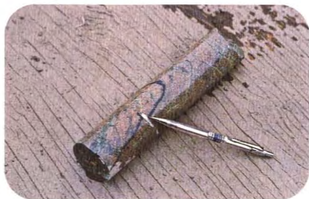
Diamond drill core containing high grade native copper in fractures and disseminated throughout the rock
