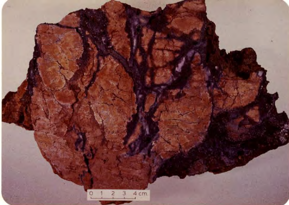
(7) Baked clay residue showing some fusion on cracks
