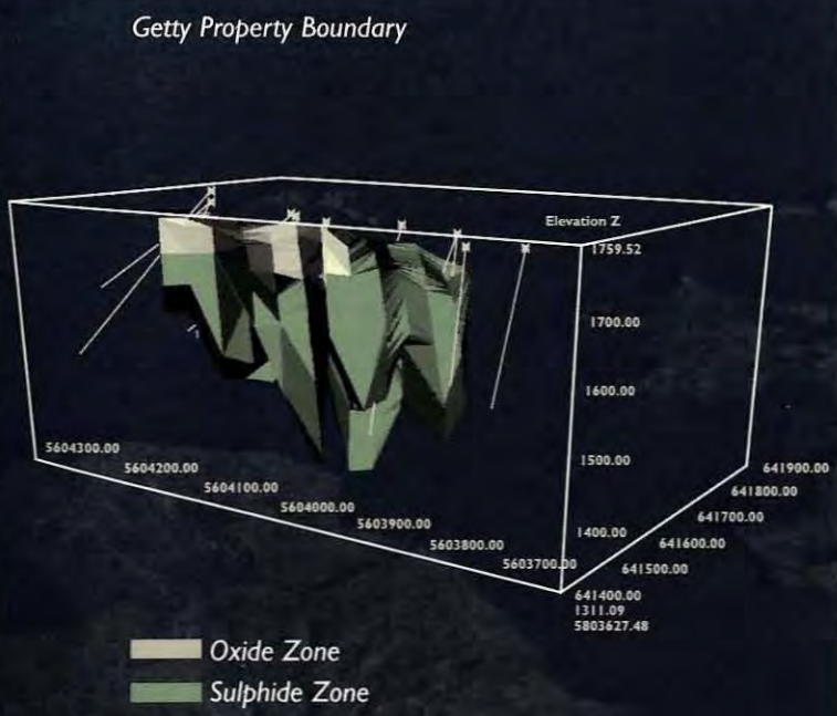
Getty North Zone Solids Model with 1996 Drilling (Watts, Griffis and McOuat Limited, 1996)
