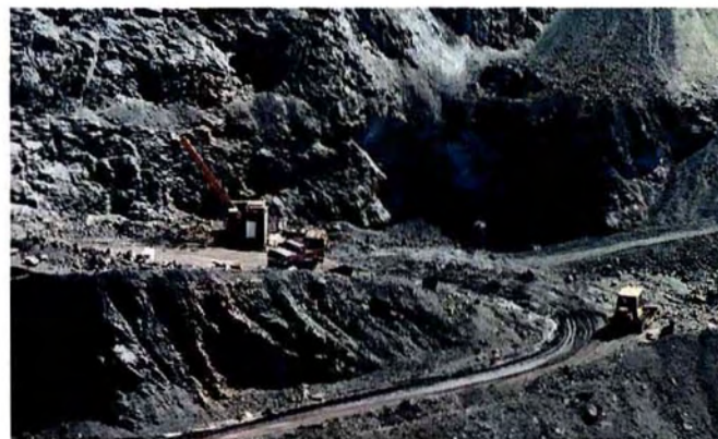
A diamond drill tests the new mineral deposit under the old Afton open-pit mine. Photo courtesy DRC Resources Corp.
