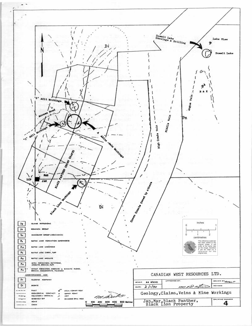
workings, cross-cutting drifting and trenching by Pioneer (1941 to 1946) have outlined mineralization at the C and B adits which returned values of 0.75 ounces gold per ton over a 23.48 centimetre width for 45.72 metres and 2.09 ounces gold per ton over 12.8 centimetres for 36.58 metres, respectively.
