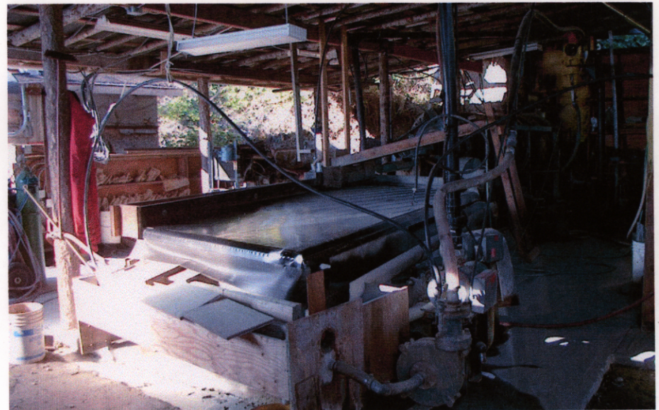
October 3, 2001 - Bob Duker's backyard pilot mill at Texada Island - gravity table
