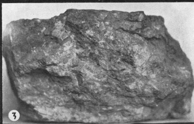
(1) Selected samples assaying from 3 to 19 ounces gold per ton. (2) Hand-picked ore, such as will be shipped direct to smelter as mined. (3) Sample from Gibson Vein measuring 10 inches wide and weighing 80 pounds—free gold visible.
