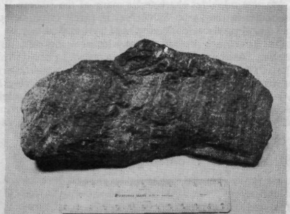
FIGURE 8(c). Stratiform ore from Myra Main Zone, with chalcopyrite, sphalerite, barite and minor galena.
