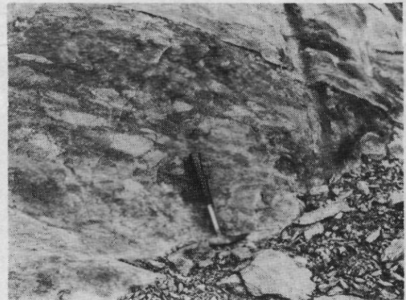
FIGURE 3(c). Monolithic breccia consisting of clasts of sericitized rhyolite? in a sericitic and pyritic matrix, found a few tens of metres south of 'G' zone. The long axes are parallel to the dip of 'G' zone. Similar rock in Precambrian volcanogenic deposits has been called 'mill rock' (Lajoie, 1977).
