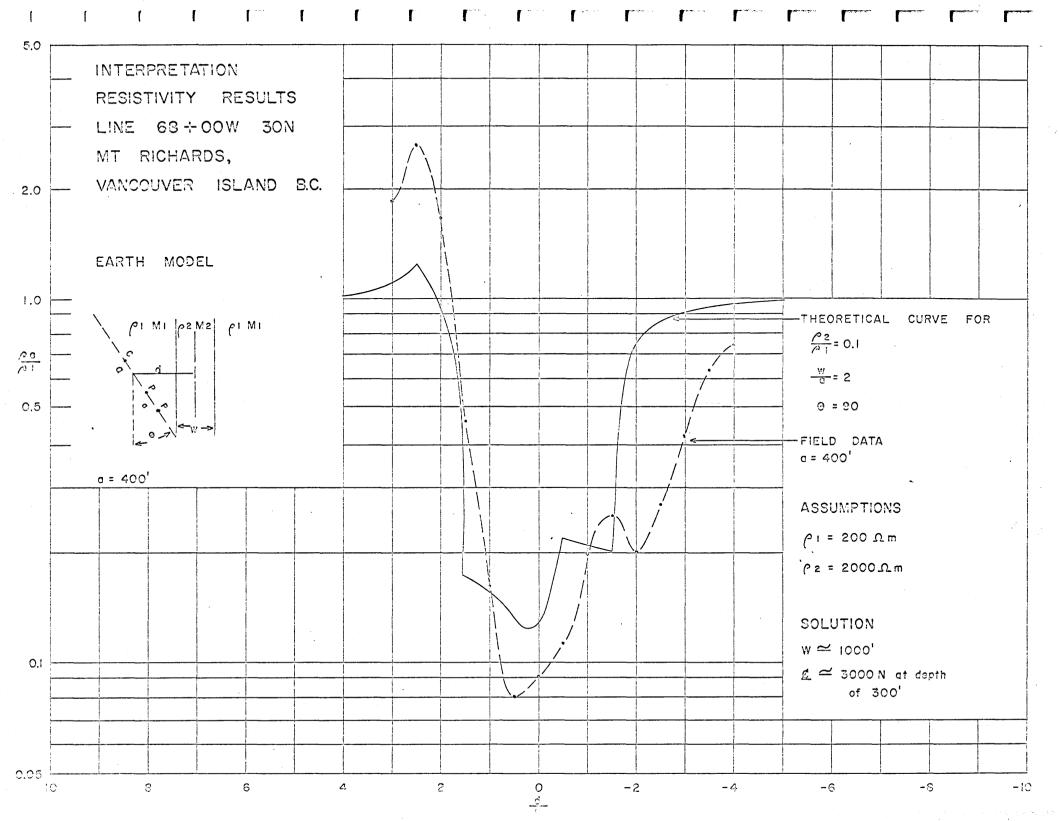
Comparison with the best fitting theoretical curve shows a dike about 1000 ft. wide centered at about 3000 ft. N at a depth of 300 ft.
